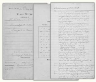
Field notes are the narrative record of the cadastral survey. They are written in tabular format and contain the detailed descriptions of entire survey process including the instrumentation and procedures utilized, calling all physical evidence evaluated in the survey process, and listing all of the individuals who participated in the work.
