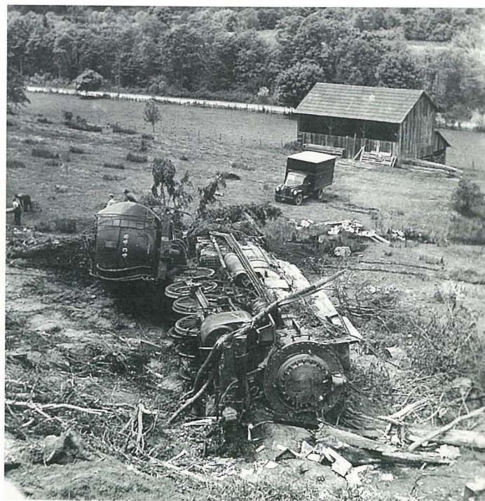
On May 7, 1943, Train 330, pulled by engine 4348, failed to negotiate a curve in Douglas County, and the locomotive and several cars derailed and plunged down an embankment. Engineer J.H. Corbett was killed in the accident, and Fireman I.L. Smith was burned by hot oil as he crawled from the wreckage. The official cause for the wreck was excessive speed.
